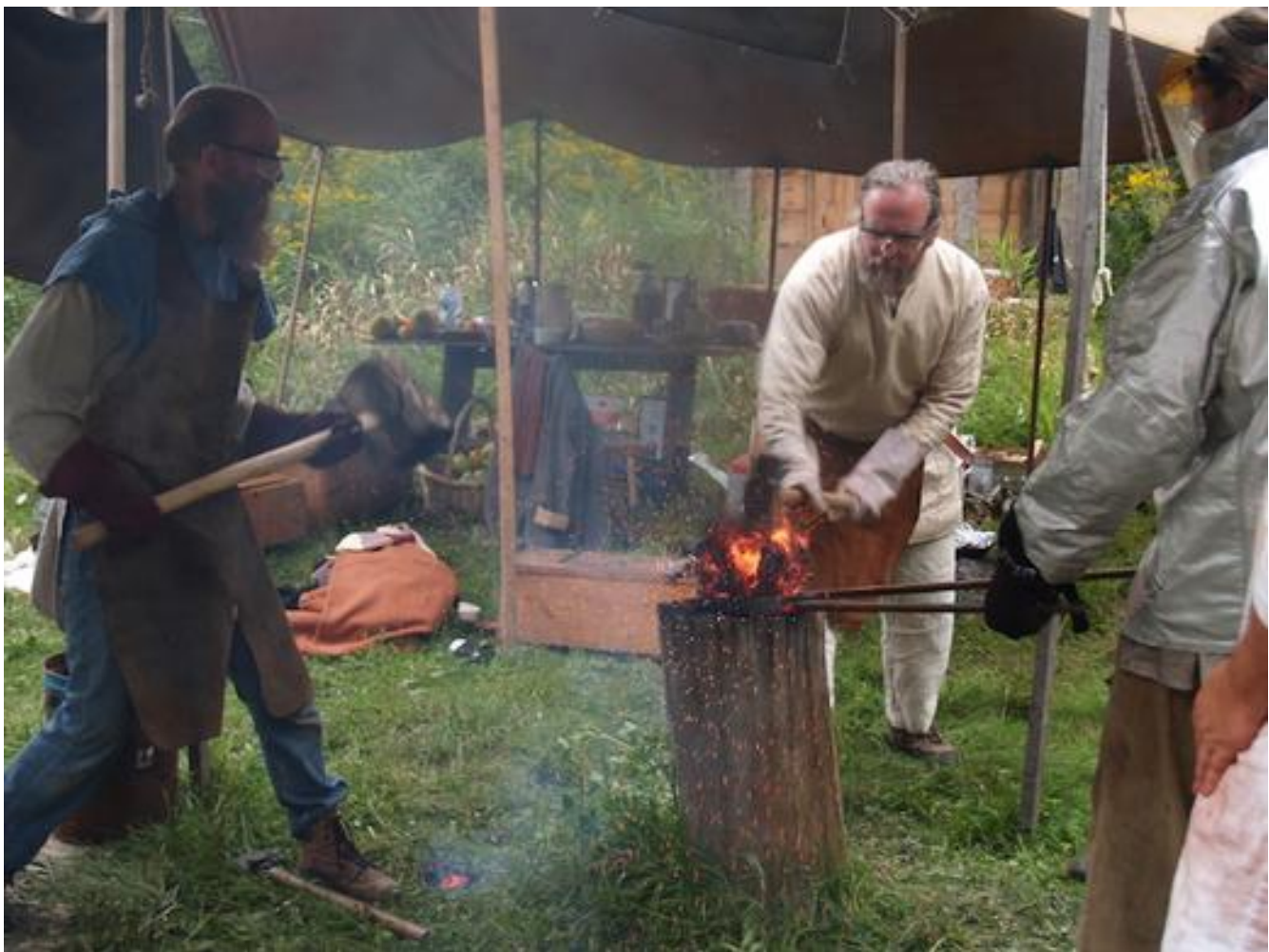
Marcus Burnham with the ‘Troll Hammer’, Richard Schwitzer with a standard sledge, Dave Cox holding. The slag shows as the darker material still encasing the hot metallic bloom core.
